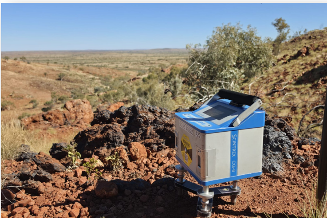
Figure 1. Gravity surveying in progress at the Pearana Prospect adjacent to manganese outcrop
